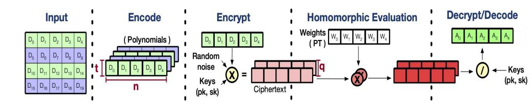
Algorithm/hardware co-design of private machine learning inference systems using cryptographic techniques such as homomorphic encryption and secure multiparty computation
